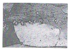
Figure 4. Optical micrograph of specimen of ferritic stainless steel type 409, deformed at an effective strain of 0,58 and at a single temperature of 870°C, showing a poorly developped substructure as well as coarse precipitates with different shapes. X300.
